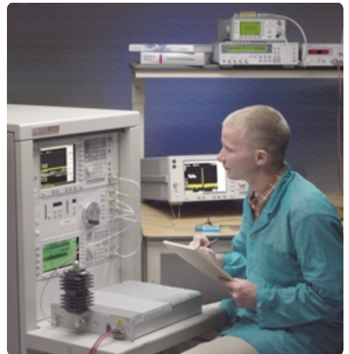
The PSA series simplifies multi-carrier power amplifier (MCPA) testing with in-channel, adjacent channel, and out-of-band measurements in one analyzer.
